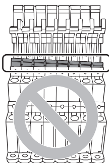
Incorrect installation Some terminals not inserted completely.
