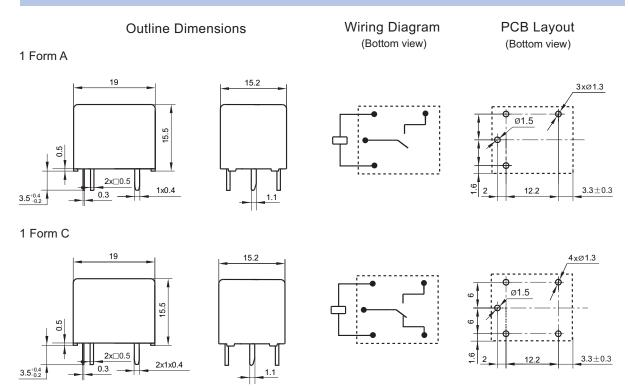
Remark:1)In case of no tolerance shown in outline dimension: outline dimension ≤1mm, tolerance should be ±0.2mm; outline dimension >1mm and ≤5mm, tolerance should be ±0.3mm; outline dimension >5mm, tolerance should be ±0.4mm.
