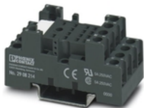
ECOR-2 relay base, for industrial relays with four changeover contacts, bolt connection, for mounting on NS 35/7,5
